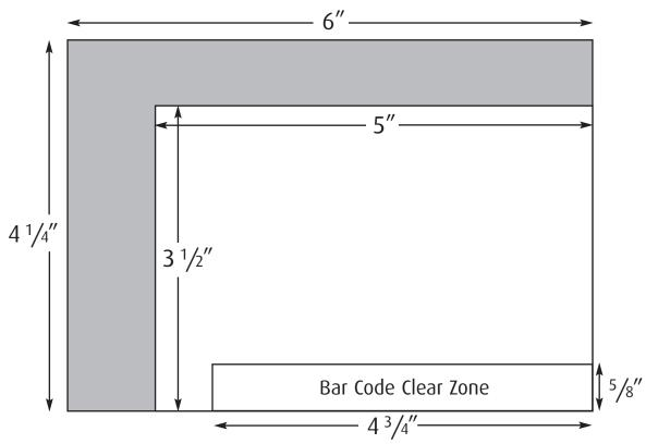
Bar Code Clear Zone is where postal bar code may be sprayed. **Do not place text in this zone.**
